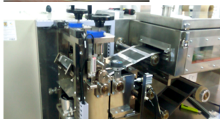
Fig. 1. A ready-to-coat cathode slurry (a); roll-to-roll processing technology using the semi-automatic electrode coating machine - intermittent coating (b)
