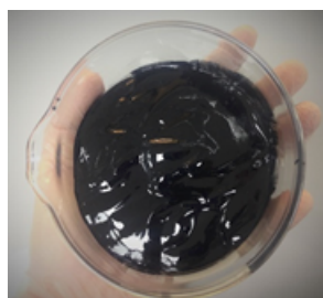
Fig. 1. A ready-to-coat cathode slurry (a); roll-to-roll processing technology using the semi-automatic electrode coating machine - intermittent coating (b)
